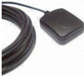
Patch Antennas are made from a flat patch internal to the antenna's housing. They can detect satellites directly overhead but cannot detect satellites on the horizon. They should be held flat for best reception.
